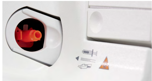
Figure 13. Sample port location.
